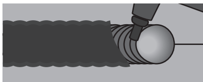
PARTIALLY CHIPPED AWAY TO SHOW WELD
